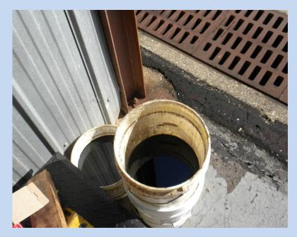
Drip bucket (good control) but they should be tightly sealed when not in use. Note the proximity to the storm drain.
